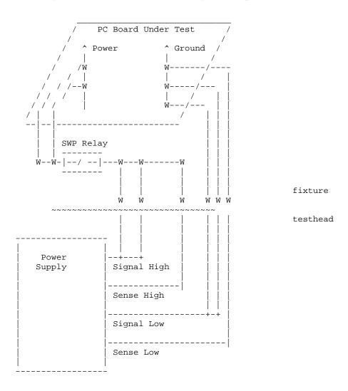
This diagram shows a positive voltage power supply; a negative voltage power supply would swap the highs and lows.
